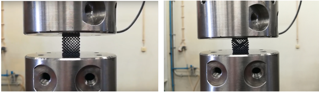
FIGURE 7.51: Mechanical testing of the specimens with the conventional honeycomb core geometry and only top and bottom face sheets, in compression.
