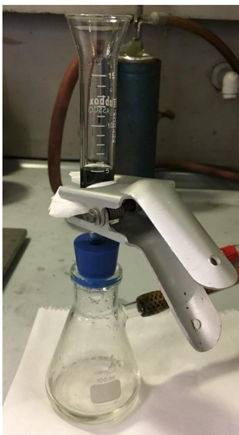
Figure A.4. Vacuum filtration step during the fabrication of supported membranes.
