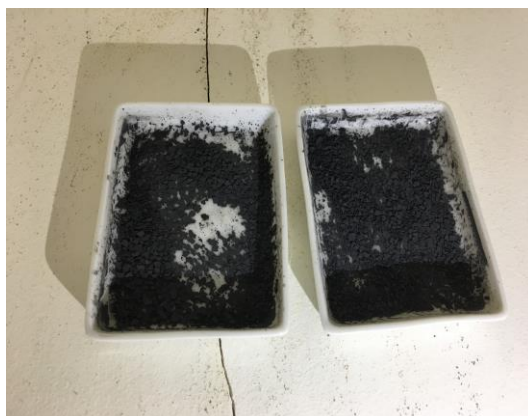
Figure A.2. Graphite oxide impregnated with melamine, after the thermal treatment in the muffle furnace.
