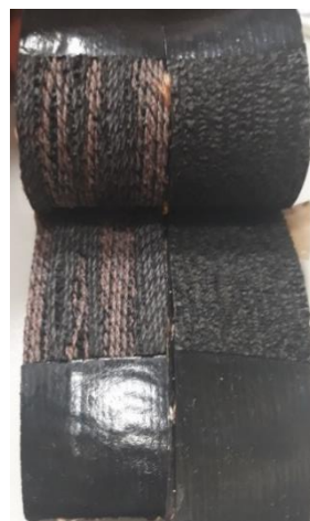
Figure 7 - Peel adhesion test result: bad result (at left) and a good one (at right).
