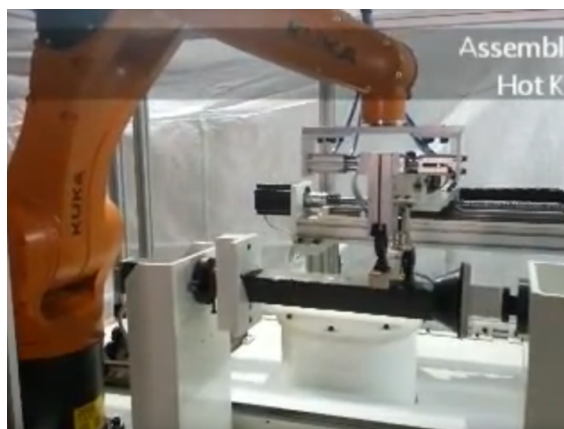
Figura 2.27: Wax pattern assembly automation [19])
