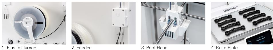
Figure 2.1: Key components in FDM 3D printing [19]
