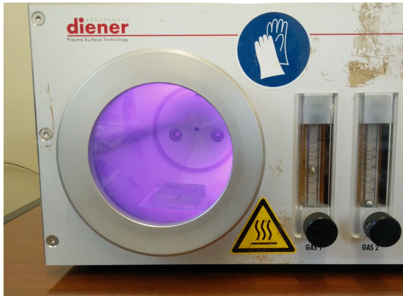
Figure 3.23: Surface treatment of PDMS in a plasma cleaner
