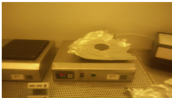
Figure 3.15: SU-8 mold soft baked onto a hotplate
