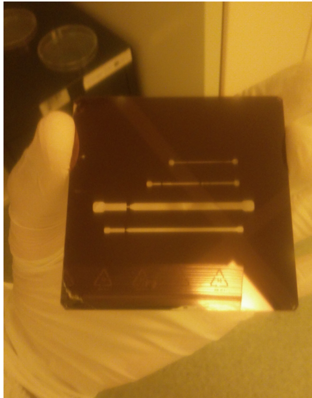
Figure 3.14: Pattern Mask fabricated with a AZ1505 photoresist
