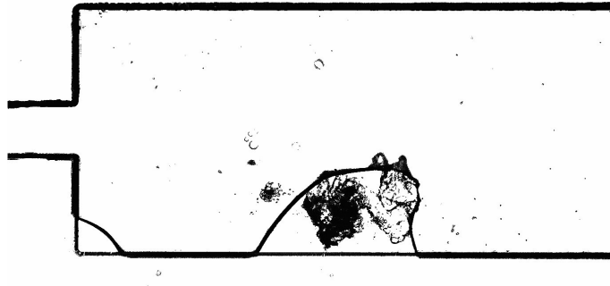
Figure 3.27: PDMS debris and air bubbles trapped inside micro-channels
