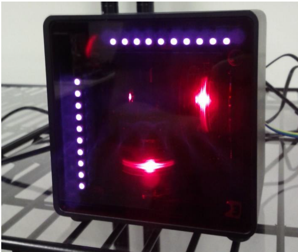
Figure 3.1: The inside of a SteamVR base station
