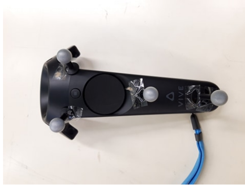
Figure 5.3: Vive controller with Optitrack markers
