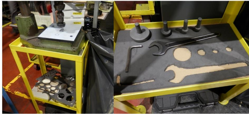
Figure 23: Shadow board (before and after).
