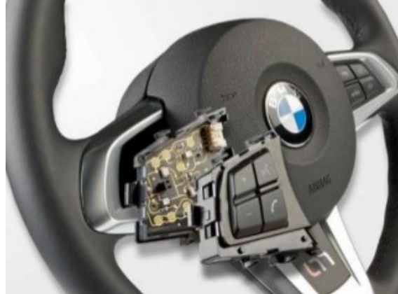
Figure 2.12: Example of an LDS automotive implementation [18].
