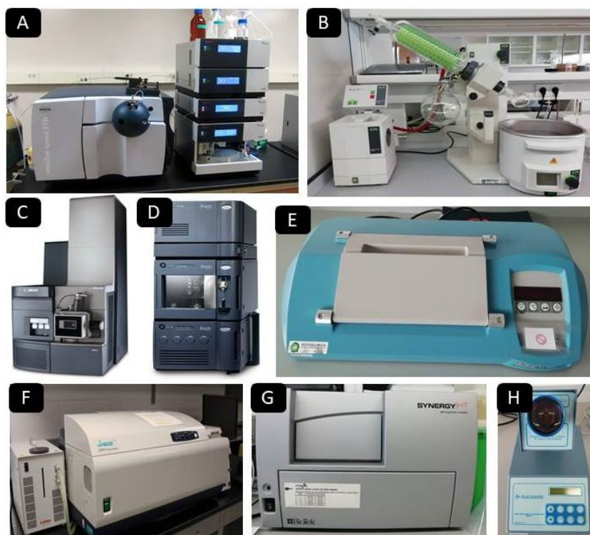
Figure 14 – Equipments used through the stage: A - Bruker AMC instrument; B - Büchi heating bath B-491, rotavapor R-210, vacuum module V-801 EasyVac and vacuum pump V-700; C - Waters Xevo QToF mass spectrometer; D - Waters Aquity UPLC system; E - ADP410 Polarimeter; F - Jasco J-815 CD spectropolarimeter and G - BioTek Synergy TM HT Microplate Reader, H - Stuart Scientific Melting Point Apparatus SMP3.
