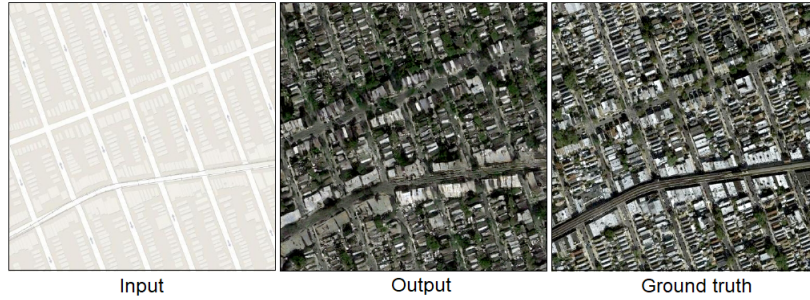
Figure 4.4: Exemplifying result for the application of the pix2pix for the generation of images from the Inria Aerial Image dataset. From left to right, the input image, the output image and the ground truth. Source: [IZZ17]
