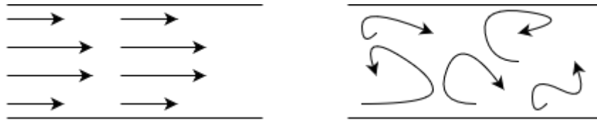
Figure 3. 5 - Schematization of laminar (left) and turbulent (right) flow regimes.
