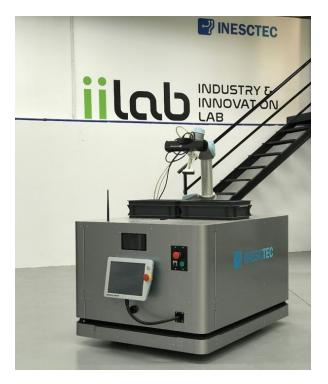
Figure 4.1: FASTEN Mobile Manipulator
