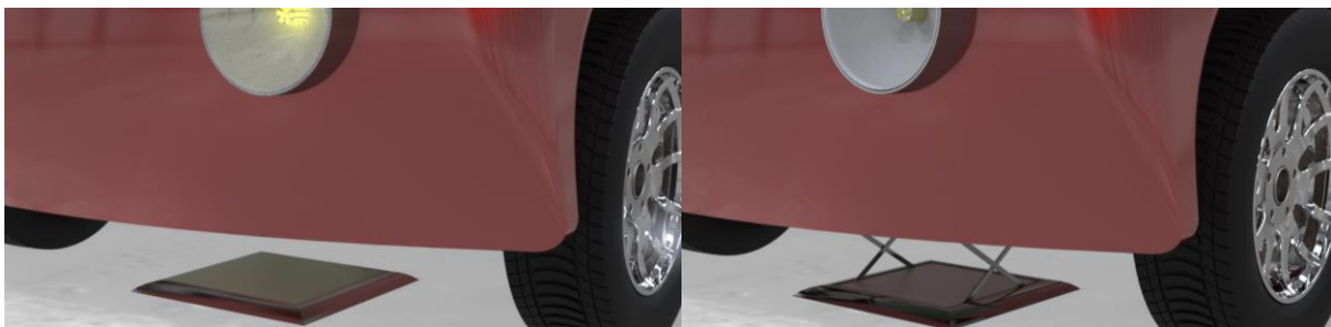
Figure 62 – Charge pad below the vehicle before and after the car turn off
