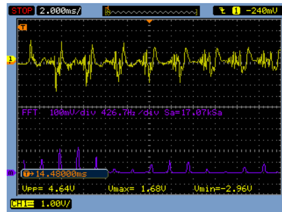
Figure 35: Amplified Piezo Result of medium pluck with FFT
