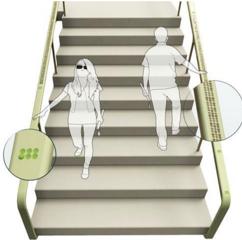
Figure 24 - Project developed by the designers Zhou Wenqiang, Bao Haimo, Jin Zhixun, Li Meiyun and Li Xinyi: staircase handrail with braille to help vision impaired users that can be used in any settings (from (Tuvie, 2018))
