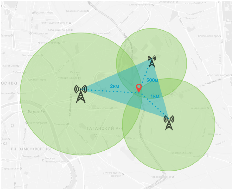
Figure 2.1: Triangulation process of a GPS system
