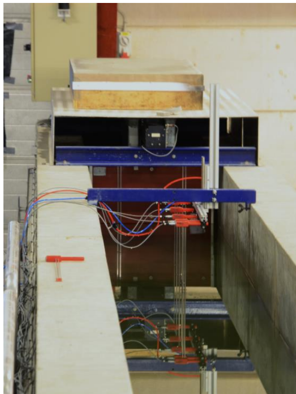
Fig. 4.6 - Wave maker and wave gauges at DHI facilities in Hørsholm (Hansen and Schlutter, 2018).
