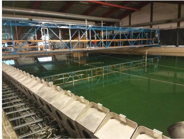
Fig. 2.7 - Wave tank at DHI facilities.
