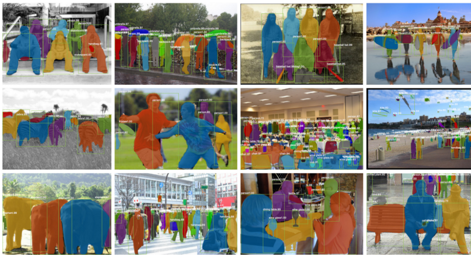
Figure 2.45: Mask R-CNN aggregates the best of the previous model by being able to segment and classify objects in an image 13
