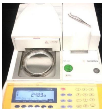
Figure 16 - Solid Content measurement device.
