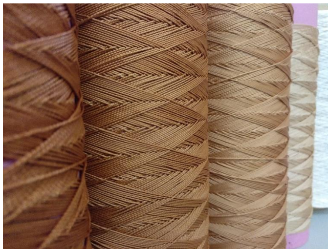
Figure 15 - Rayon cords with different percentages of Solid Content.
