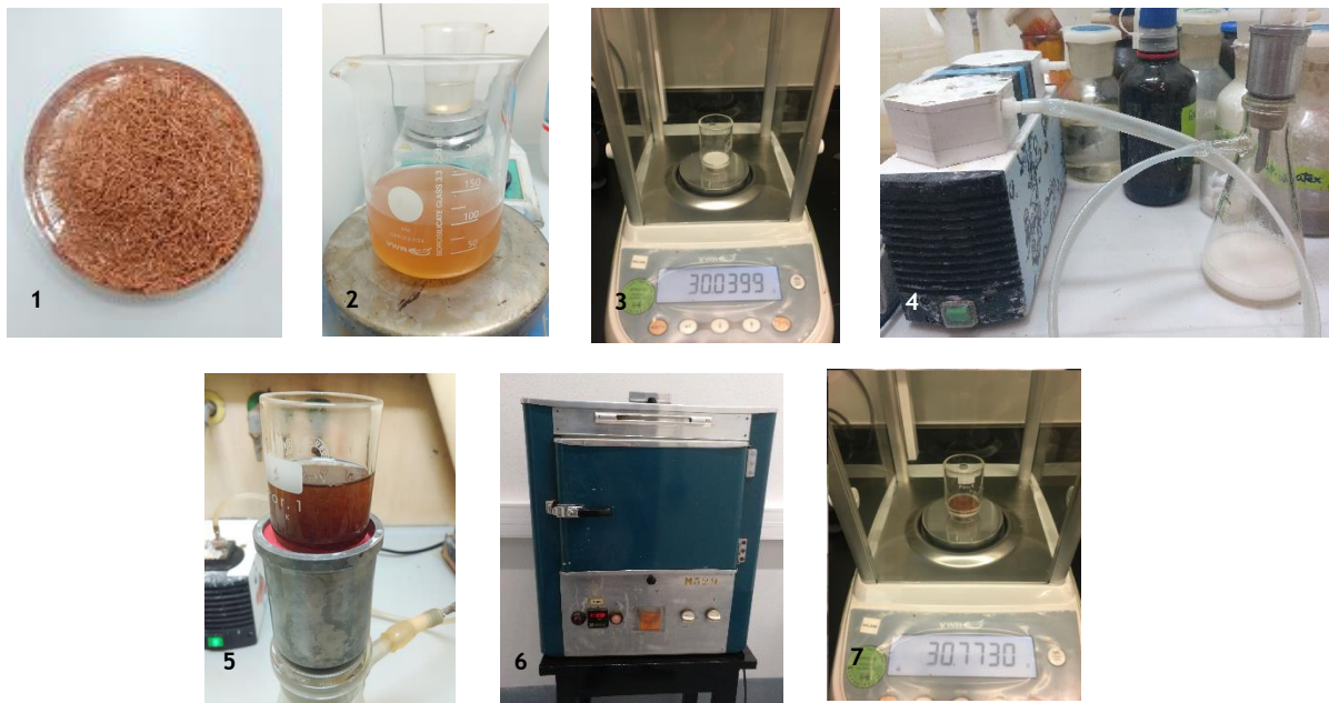
Figure 11 - Wet-Chemical method procedure for Rayon.
