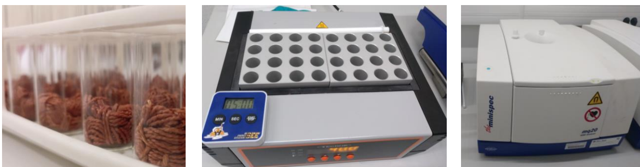
Figure 14 - Procedure of the time optimization test. On the left the samples are represented, on the middle the heating support and on the right the TD-NMR equipment.
