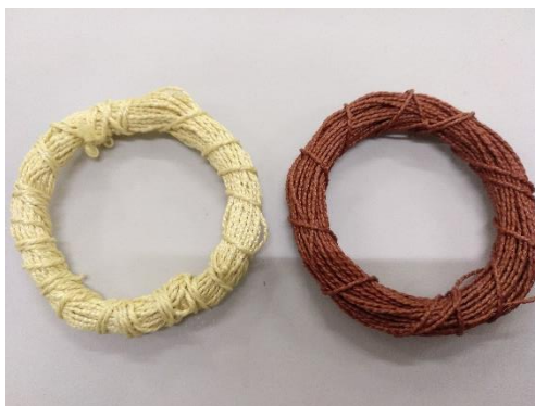
Figure 12 - Representation of the samples for Weighing method: greige cord on the left and dipped on the right side.
