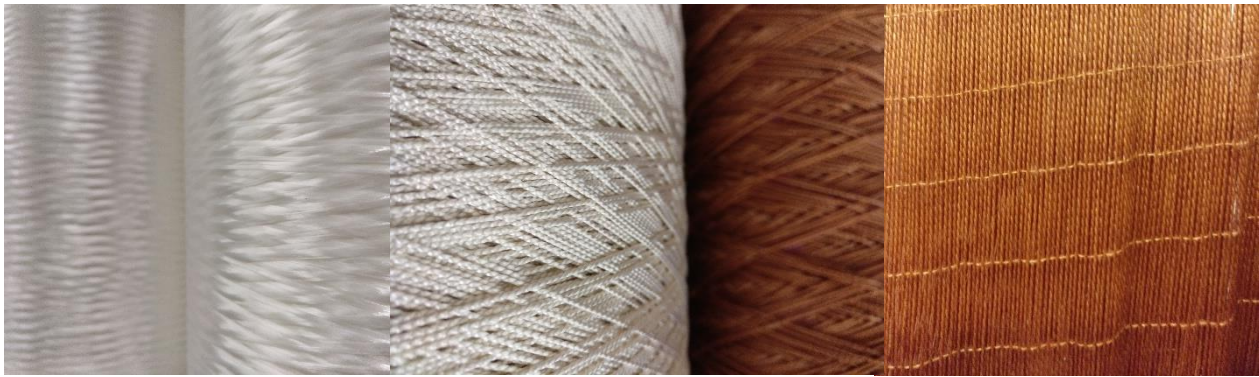
Figure 2 - Example of a yarn, cord and fabric, from greige to dipped form, named from left to right.
