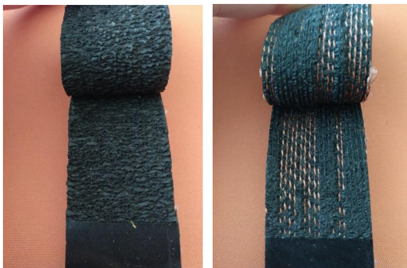
Figure 7 - Example of a peel adhesion test results: showing a good result, on the left, and a bad one on the right.
