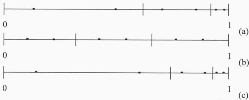
Figure 5.16 (a) isovolumetric, (b) equidistant, and (c) user defined, discretization of the spatial particles domain, \rho , for N_{er}=3 with two collocation points in each subinterval.
