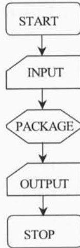
Figure 2.6 Flow diagram of computer program to numerically solve the models presented in Table 2.4. The subroutine PACKAGE refers to the package used depending on the type of problem to be solved.
