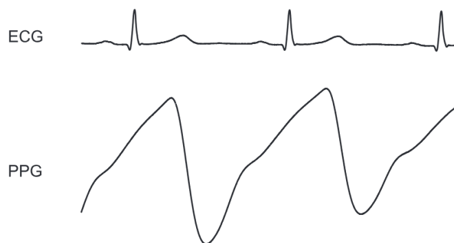
Figure 2.4: Comparison between ECG to the corresponding PPG
