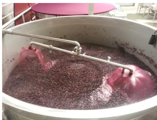
Figura 14 - Cuba com pumping over
