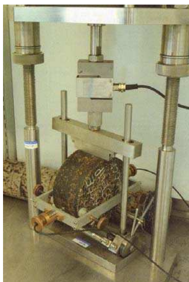
Figura 3.35 – Equipamento ITT ( Indirect Tensile Tester ) (Shell, 2003)
