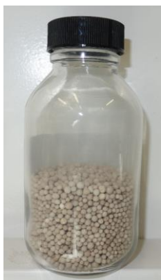
Figure 3.1 - Photography of the catalyst particles of Pd/Al 2 O 3 .
