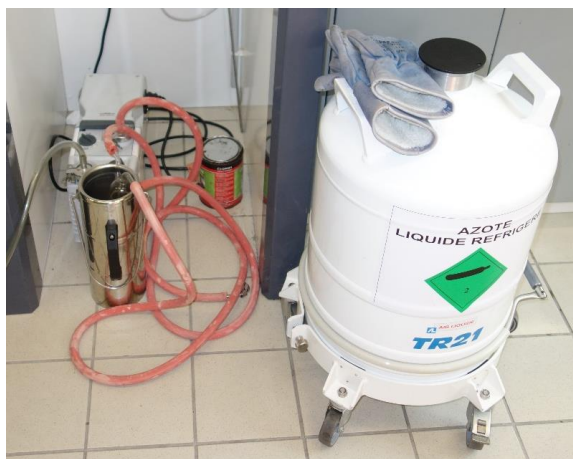
Figure 3.5 - Vacuum pump and liquid nitrogen container.
