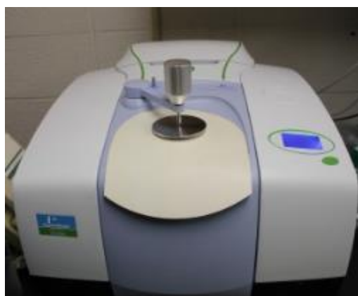
Fig. 9 - Fourier transformed infrared spectroscopy in attenuated total reflectance mode (ATR-FTIR) equipment.
