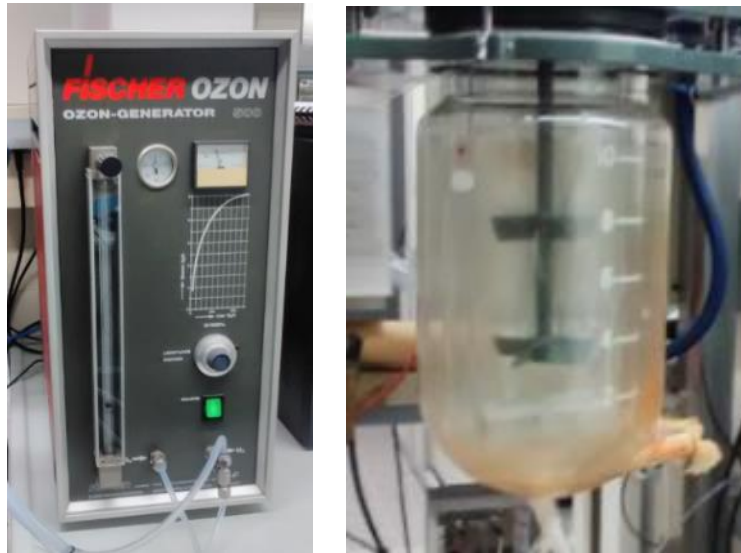
Fig. 14 - Ozone generator equipment (left) and 10 L bioreactor (right) at CeNTI.
