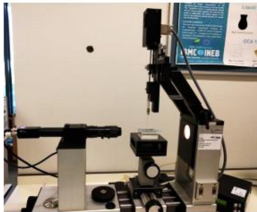
Fig. 6 - Goniometer equipment set up for captive bubble measurements.
