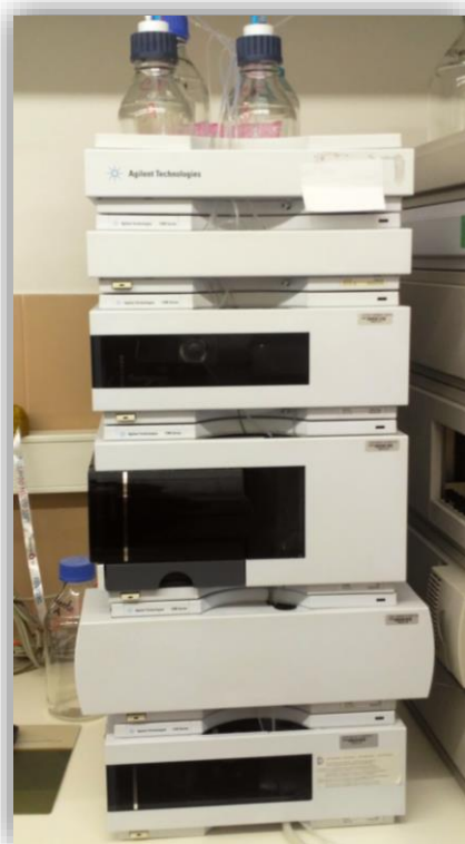
Figura 10- HPLC 1200 Agilent, com detetor DAD
