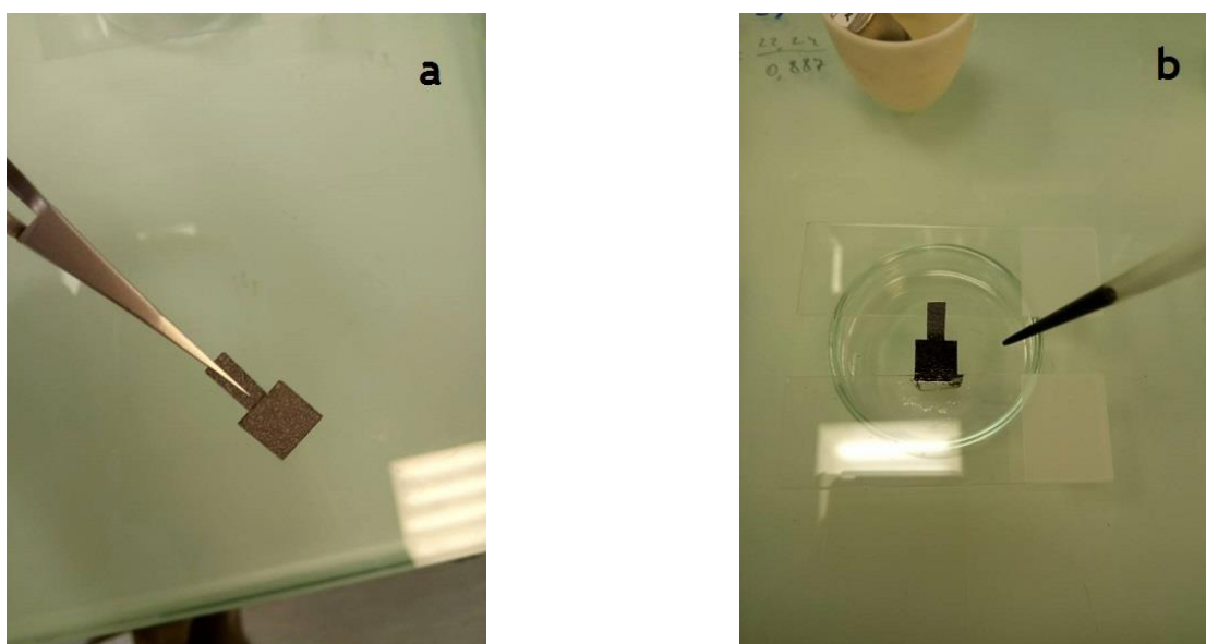
Figure 11 - Image of carbon paper before (a) and after (b) the electrocatalyst immobilization
