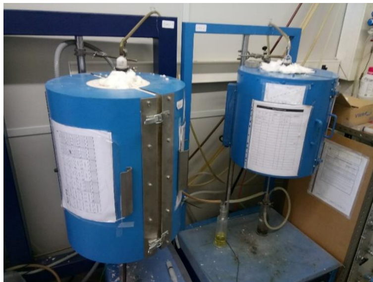
Figure 29 - Ovens from the Laboratory of Catalysis and Materials in FEUP used for the reduction of materials in hydrogen
