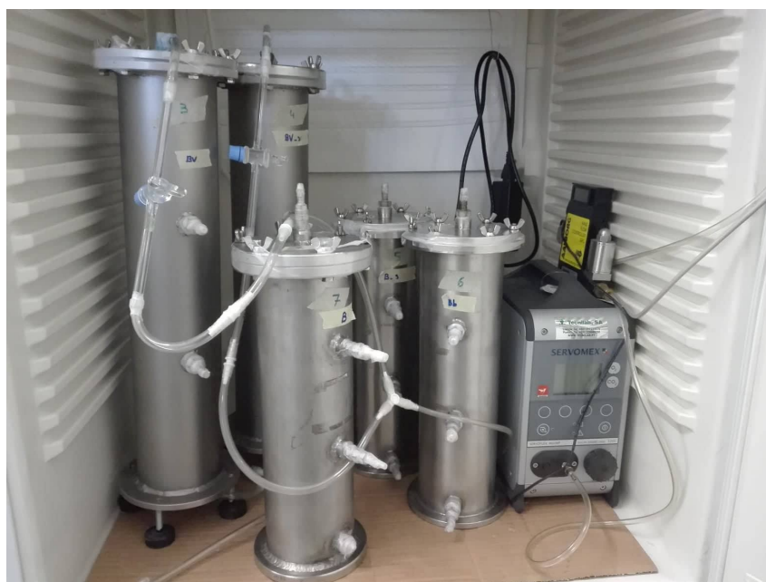
Figure 3.10: Bioremediation and Bioventilation assays setup
