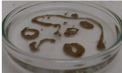
Figure 32. Printing trial of the 3% w/v PET and 10% w/w GO solution using TFA/water (1:3) as coagulation bath, a 410 \mu m dispensing tip and a flow rate of 0.5mL/h.
