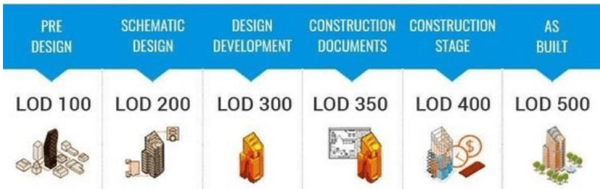
Figure 3.LOD levels and project stages. Source:[22]
