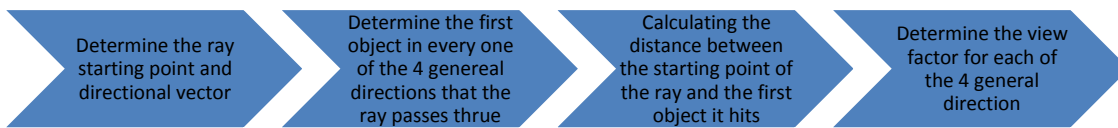
Figure 39. Ray Tracing methodology used to determine the View Factor.
