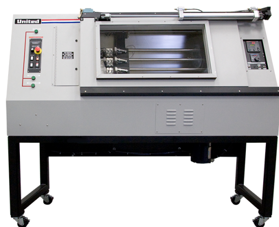
Figure 2.6: United Testing's multi-station UTM [15].
