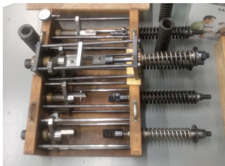
Figure 2.10: ADFEUP's spring testing apparatuses.
