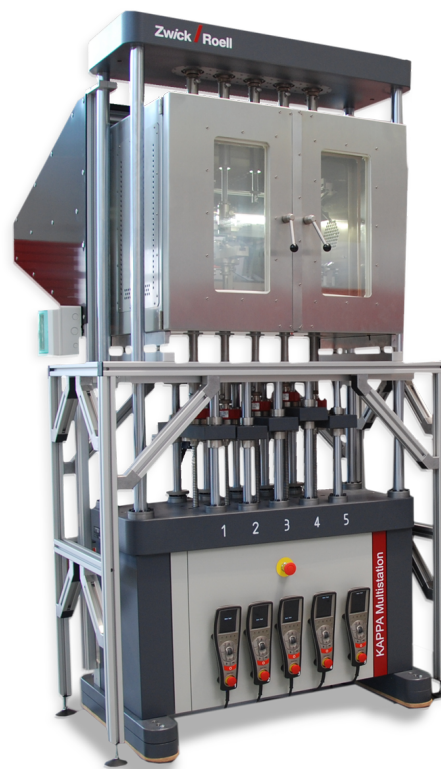
Figure 2.7: Zwick's multi-station creep testing machine [16].
