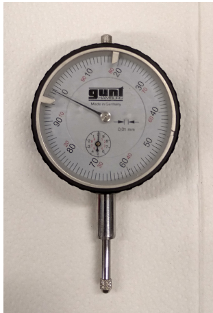
Figure 2.11: A mechanical indicator used to monitor changes in the specimens' length.
