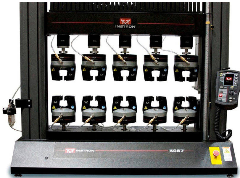
Figure 2.8: Instron's multi-station UTM [17].
