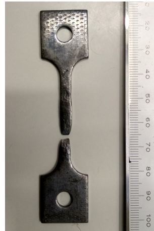
Figure 5.6: A lead specimen after testing.
