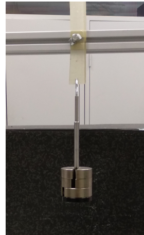
Figure 2.12: Creep test using weights.
