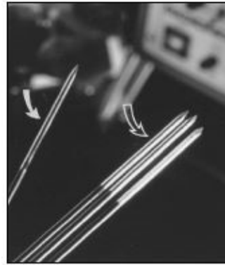
Figure 2.15: Picture representing the configuration of the tips with cooling system of the RF electrodes developed by Radionics [9].
