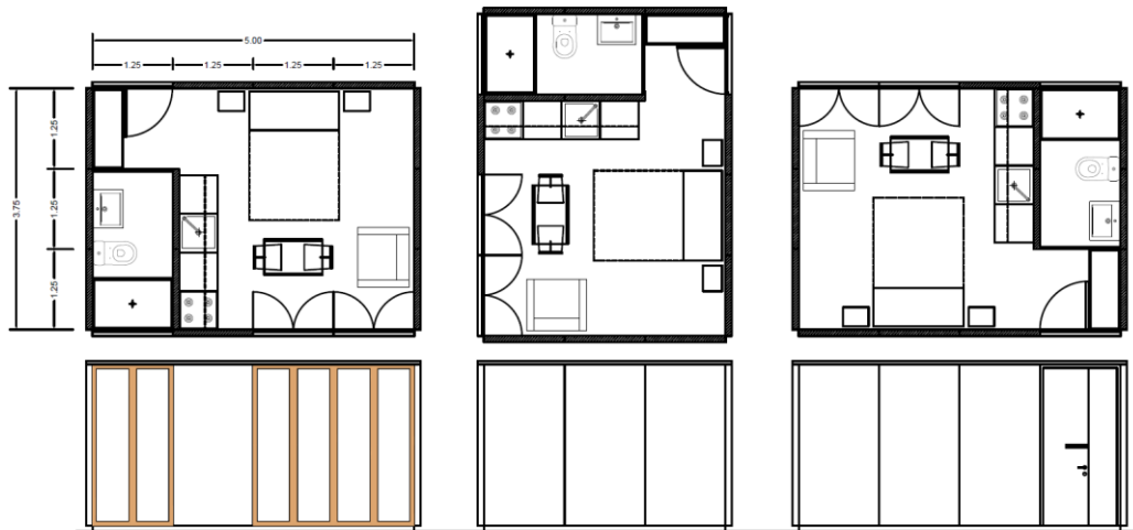
Figure 3 Possible configurations for T0 apartments using Patent 107465(PT) (3)
