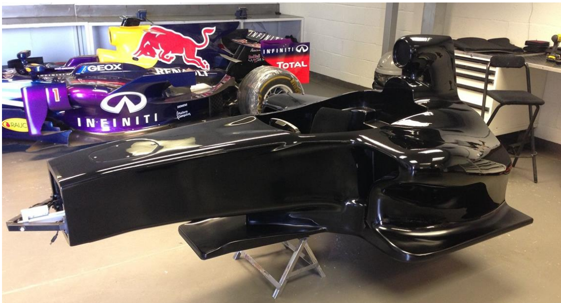
Figure 15 Example of a monocoque structure (F1 chassis) (10)
