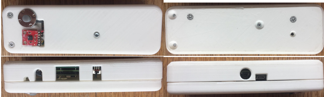
Figure 3.5: Bottom, top and side views of the second prototype. On the bottom view, the two sensors can be seen. On the side views, both buttons, the earphones, the SD card and the micro USB for charging outlets can be observed.
