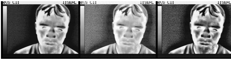
Figure 2.3: a) Thermal Image (taken from public IRIS dataset) b) Histogram-equalized image c) CLAHE image. It can be noticed that b) still suffers from low contrast, while c) is a much higher contrast image
