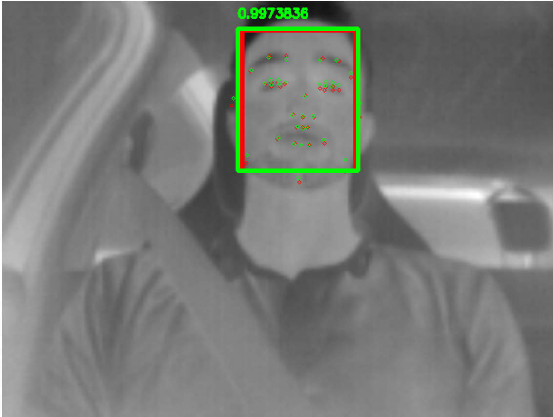
Figure 4.5: Facial landmark predictions: in green our predictions, and in red the ground truth keypoints
