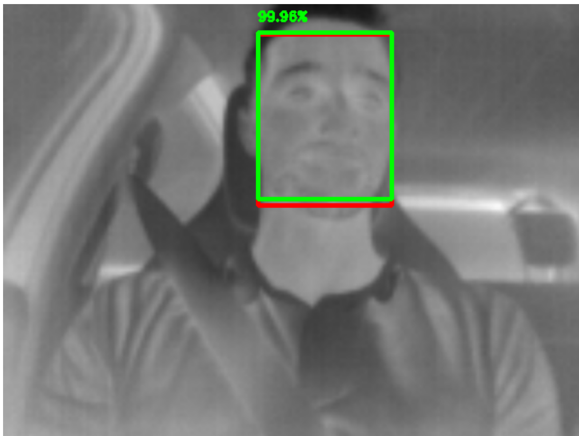
Figure 4.2: Example images. In green, the bounding box prediction from our system, and in red the ground truth. On top of the boxes the predictor's confidence is shown.
