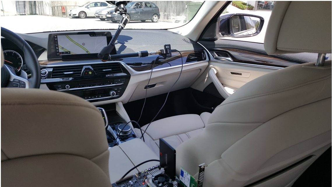
Figure 3.5: Camera setup view from inside the car.
