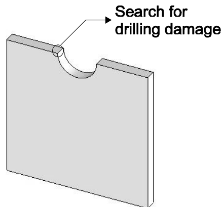
Figure 5-3: Specimen used for microscopic inspection
