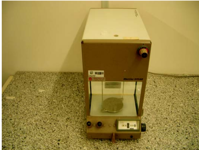
Figure 5-38: Weighing device for the determination of absorbed moisture
