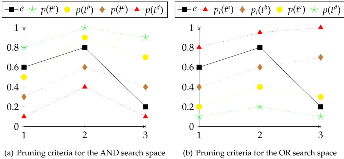
Figure 4.2: Pruning criteria for AND and OR search spaces. The x-axis contains three examples  $i = \{1, 2, 3\}$  and the y-axis represents probabilistic values ranging from 0 to 1. Four theories' prediction values  $p(t^a)$ ,  $p(t^b)$ ,  $p(t^c)$  and  $p(t^d)$  are depicted in different colours and markers. Example values are depicted as black squares
