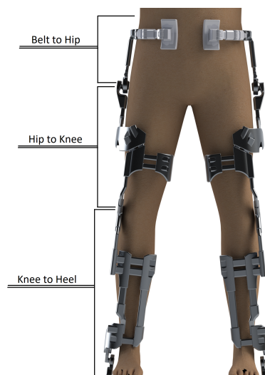
Figure 3.7: Render of the full exoskeleton frame. The components are divided into 3 sections: Belt to Hip in section 3.3.1, Hip to Knee in section 3.3.2 and Knee to Heel in section in 3.3.3
