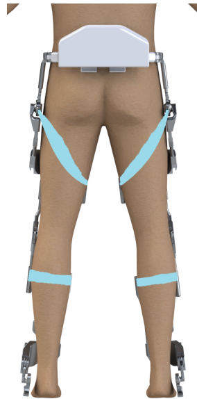
Figure 3.36: Render of the exoskeleton with the planned fastening belts highlighted in blue.
