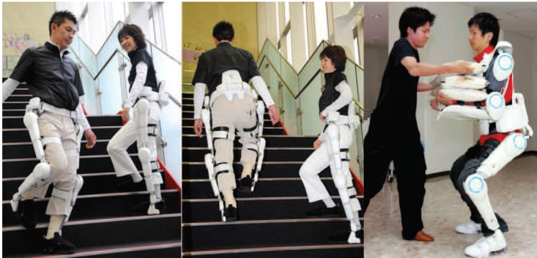
Figure 2.3: Still pictures of promotions videos of the HAL "Body Suits". On the left and center, the lower limb version showing the ability to climb stairs. On the right, the full body version assisting the wearer in holding a heavy weight.
