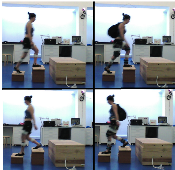
Figure 4.7: Pictures of the female subject performing stair trials with normal clothing on the left and attached weights on the right.
