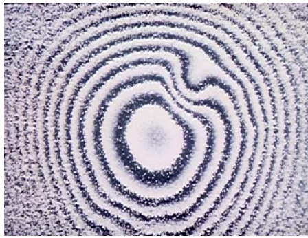
Figure 2.10 - Defect in a composite plate [31]
