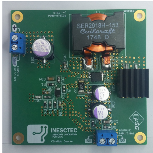
Figure 4.2: Production PCB of the boost converter
