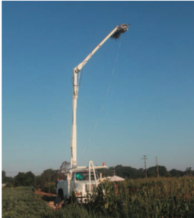
Figure 2.6: ComRAD microwave instrument system - an example of a truck-based scatterometer.
