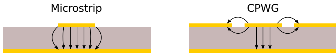
Figure 2.10: Illustration of the electric fields in a Microstrip Line and in a CPWG Line.
