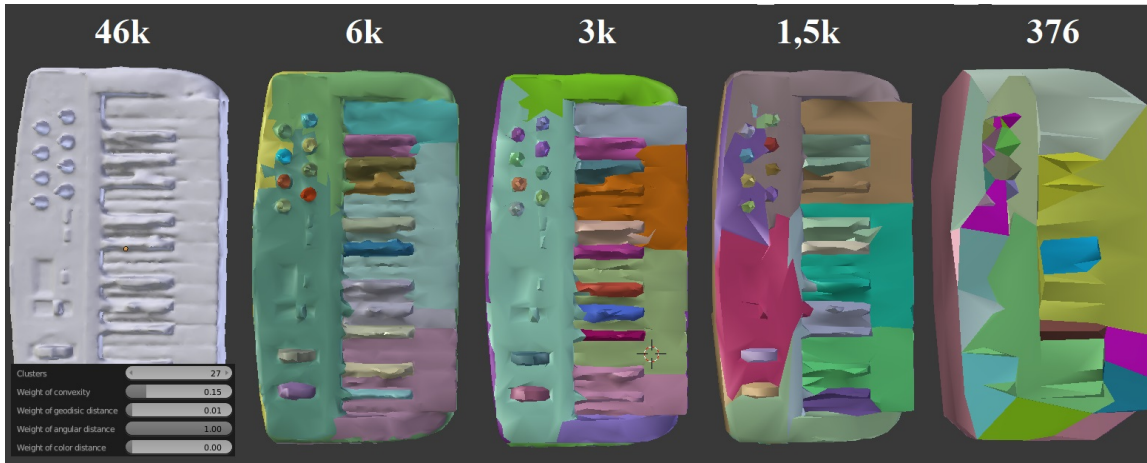
Figure 5.5: Automatic segmentation focused on angular distance over different LODs using 27 clusters.
