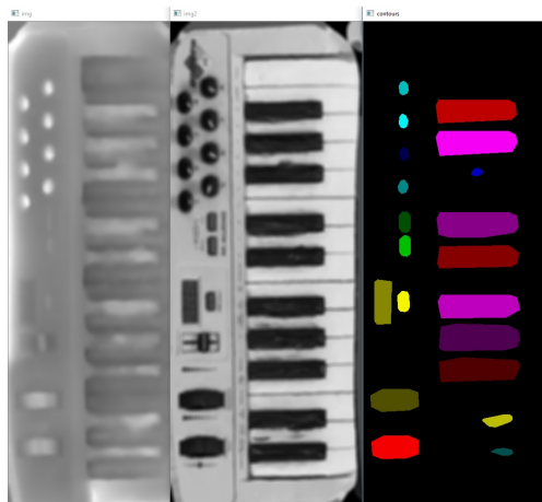
Figure 4.17: Segmentation from retopologized model displacement and grayscale color textures.
