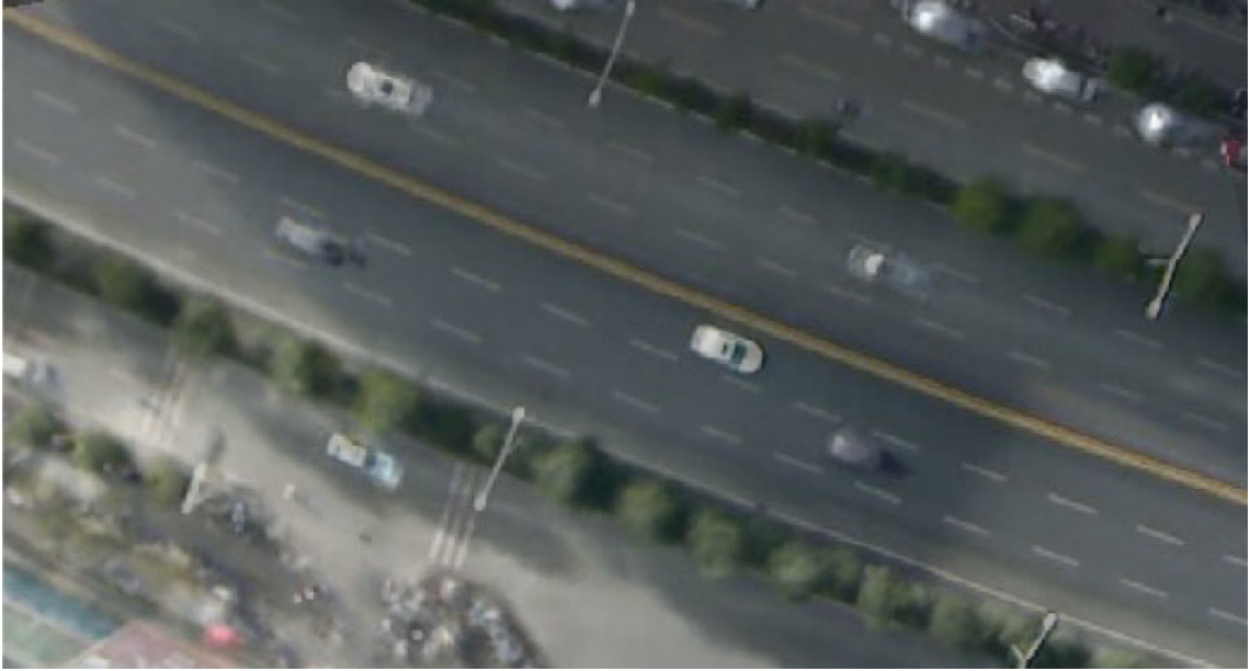
Figure 2.8: Fusion between RGB and thermal image (weight = 0.5). Notice the brighter spots corresponding to the heat emitted by the vehicle engines, mainly visible in the top right corner. (Adapted from [JLL + 17])
