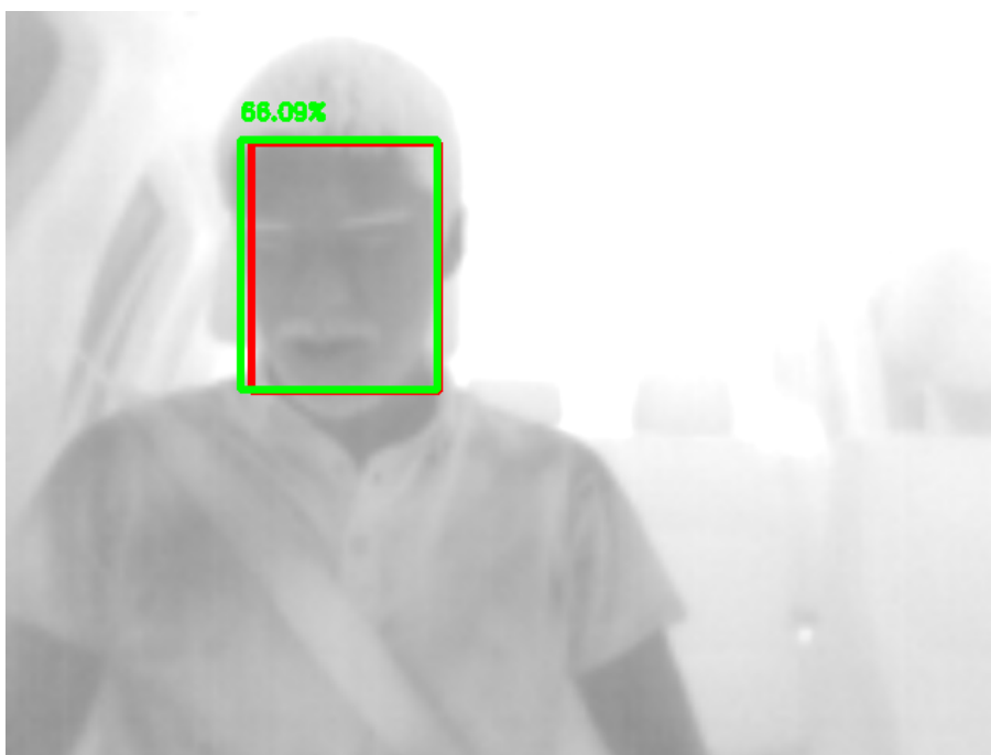
Figure 4.4: Example of a successful face detection with a high ambient temperature. The red bounding box represents the ground truth and the prediction bounding box is drawn in green together with the confidence value (66.09%).
