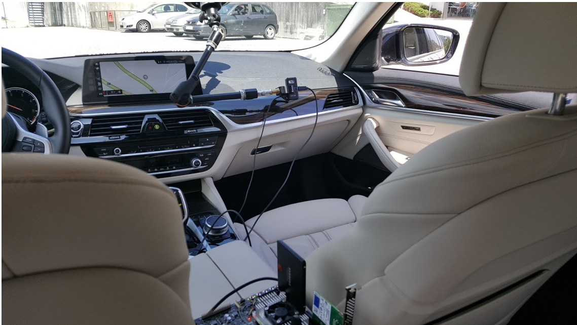
Figure 3.1: Example capturing setup inside a test vehicle. The camera is placed in front of the right front seat and is fixed in position with a folding arm.
