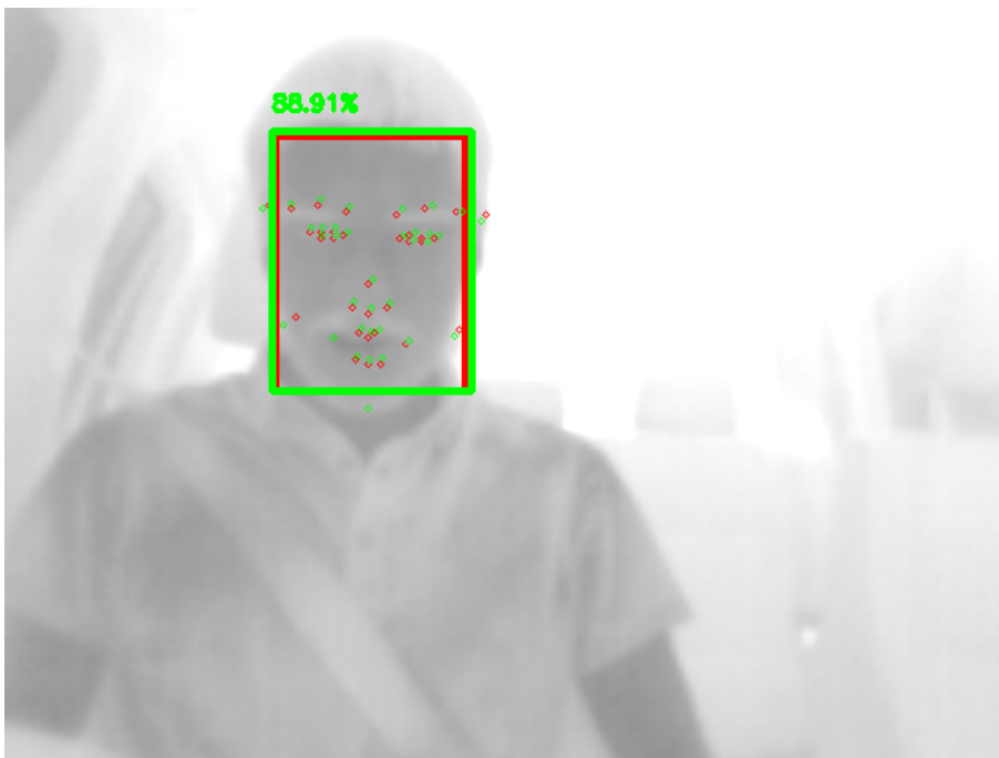
Figure 4.6: Example of a landmark detection with a high ambient temperature. Red represents ground truth and green corresponds to the predictions of the face detector and the facial landmark detector.
