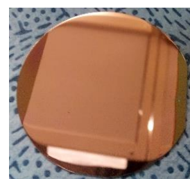
Figure 3.5 - \text{SiO}_2/\text{Si} wafer coated with Cu by sputtering.
