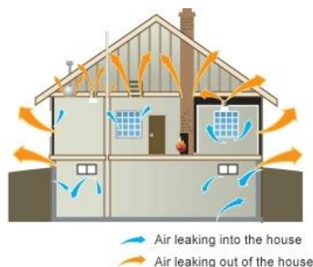
Figure 1 - Air leakage in a common house. Extracted from [33].
