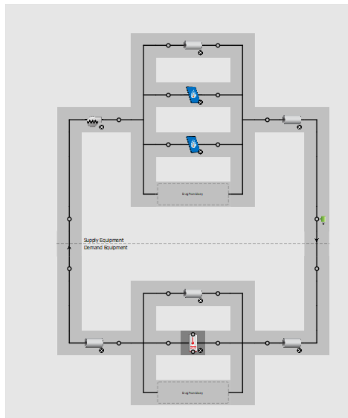
Figure 48 - Supply loop to storage tank for indoor heating.
