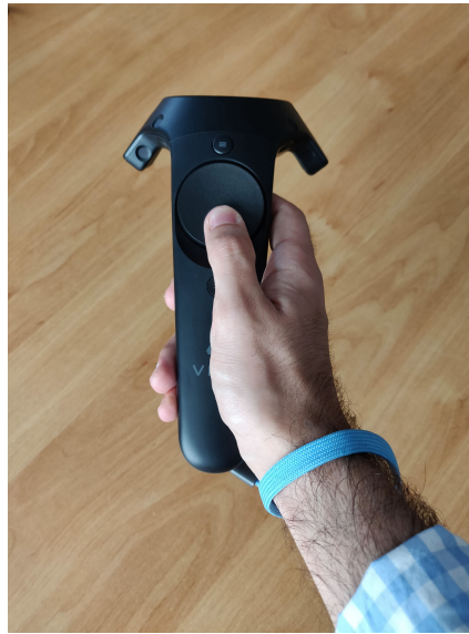
Figure 4.13: Controller with touchpad being pressed. In order to move the avatar, the touchpads on both controllers must be pressed while, at the same time, moving them in a swing-like movement.
