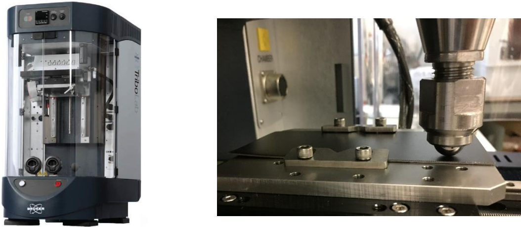
Figure 15 - Tribometer, at left ("Bruker"). Plate on ball test, at right.
