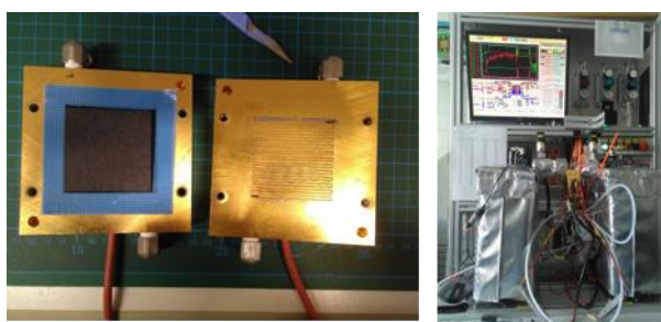
Figure 10 - Assembly of the MEA in the bipolar plate (left) and the test bench (right).
