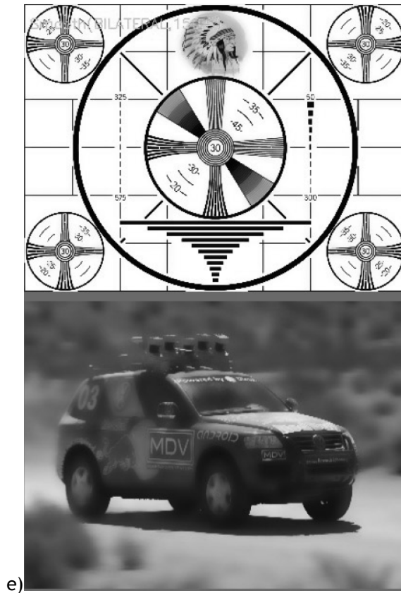
Figure 15: Different types of smoothing transformations applied to two images: a) original images; b) average smoothing; c) median blurring; d) Gaussian blurring; e) bilateral smoothing [15]
