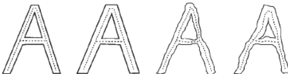
Figure 10: Use of thinning to regularize character shapes. Here, character shapes of different limb widths—or even varying limb widths—are reduced to stick figures or skeletons. Thus, irrelevant information is removed and at the same time recognition is facilitated. [13]
